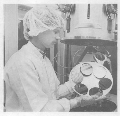
JOHN McBRAYER (6224) demonstrates the loading of silicon disks into the metal evaporator for metal deposition in the new Photovoltaic Device Fabrication Lab. Dedicated earlier this month, the lab is fully equipped to process solar cells from their beginnings as silicon disks to their final testing and packaging as module-ready cells. Reliable cell processing techniques developed in the lab will be transferred to the US photovoltaic industry.
